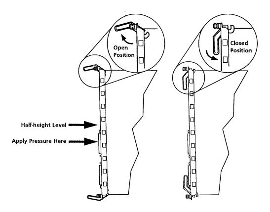
Figure 2-2. ONcore Module Ejectors
